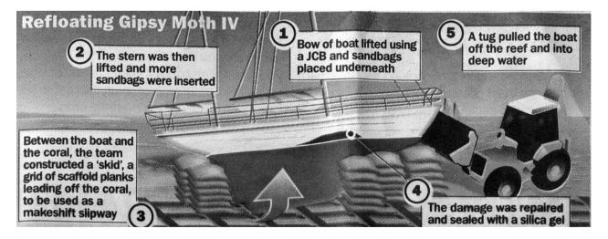
The digger lifted the boat, sandbags were placed beneath the hull and a plank slipway built to the edge of the reef. Meanwhile the hull was patched up while a nervous watch was kept on the weather. This is the season of tropical storms and there was every chance that the famous craft would be pounded to pieces. But the gods were kind.
