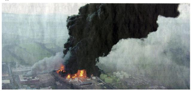
At 1900 hours on 10<sup>th</sup> December 2005 operators at the *Buncefield Oil Depot* began filling *Tank 912* with 20 000 cubic feet of petrol an hour. That is a bit faster than your run-of-the-mill petrol pump. By 0300 hours the tank was about three-quarters full. At this point the fuel level gauge stuck. Why it did so seems to be anybody's guess.
