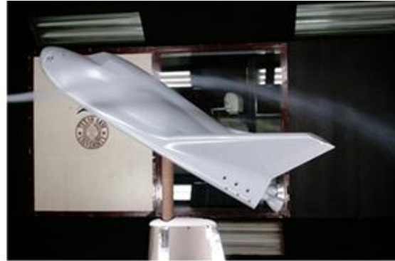
A Scale Model of the Dream Chaser® Completed Aerodynamic Testing at the Texas A&M Low-Speed Wind Tunnel.
